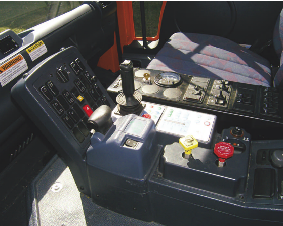
A small rocker switch below the paddle-like gear selector lets the driver pick Auto or Manual mode for the transmission's Electro Automatic Shift.
